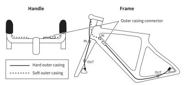
\*If you want to put the outer connector inside the frame, you must have a hole of 6.2mm or more.
