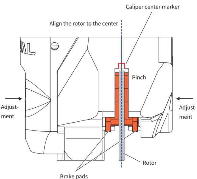
To operate the pad adjustment screw, refer to "5-1. Brake Pad Clearance Adjustment". When Centering process is done, tighten fixing bolts for caliper to the frame with certain torque.
