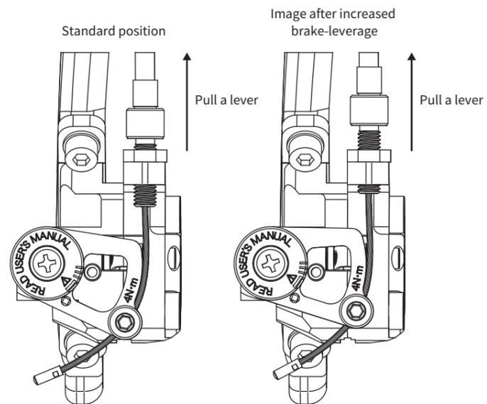
\* The standard position depends on the adjustment of the brake pad clearance.
