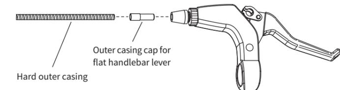
For flat handlebar, it is recommended to use only the hard outer casing, but if the rebound is too strong and you see bad effects on your handling, use the soft outer casing as well as the drop handlebar.
