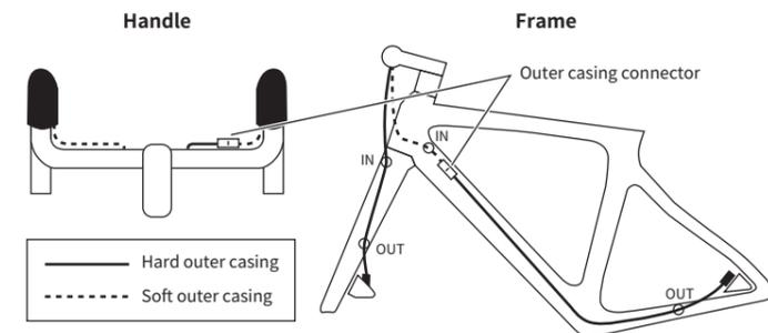
\*If you want to put the outer connector inside the frame, you must have a hole of 6.6mm or more.
